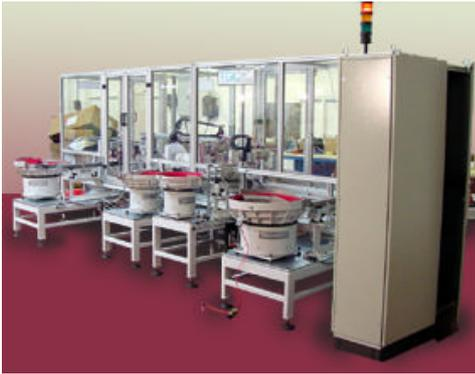
The facility is completely guarded with aluminium extruded frames and clear guard panels. All of the openings for the bowl feeders are outside the guarded area, allowing the operator to top up the bowls without stopping the machine. The deposit point for the assembled and tested product is also outside of the guarded area. The carton filling system also has an automatic carton change facility.
